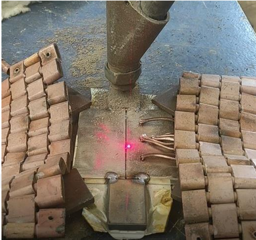
Figure 5.10. Submerged arc welding beginning of process
