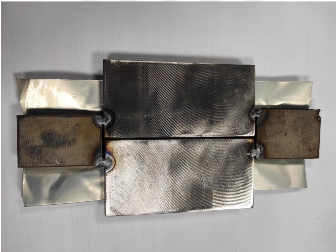
Figure 5.1. The photo of test plate prepared for welding
