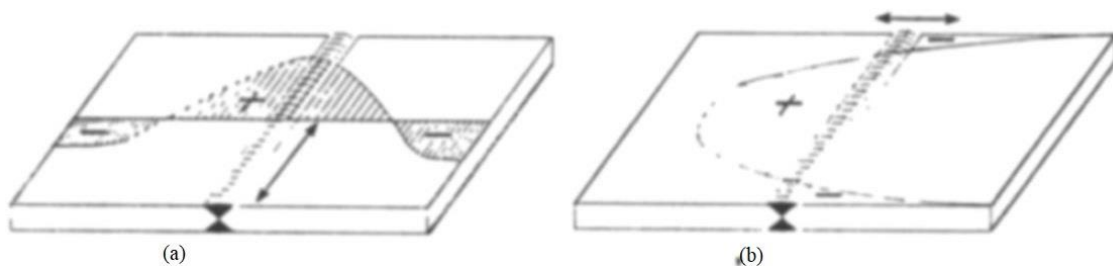
Figure 2.7. Residual stress distribution (a) longitudinal (b) transverse (Croft D.N., 1996)
