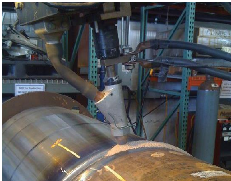
Figure 4.4. A pipe welded with SAW (Singh, 2021)
