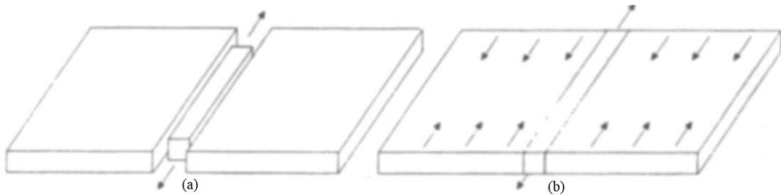
Figure 2.6. Effects of restraint on weld metal (a) Unfused (b) Fused (Croft D.N., 1996)
