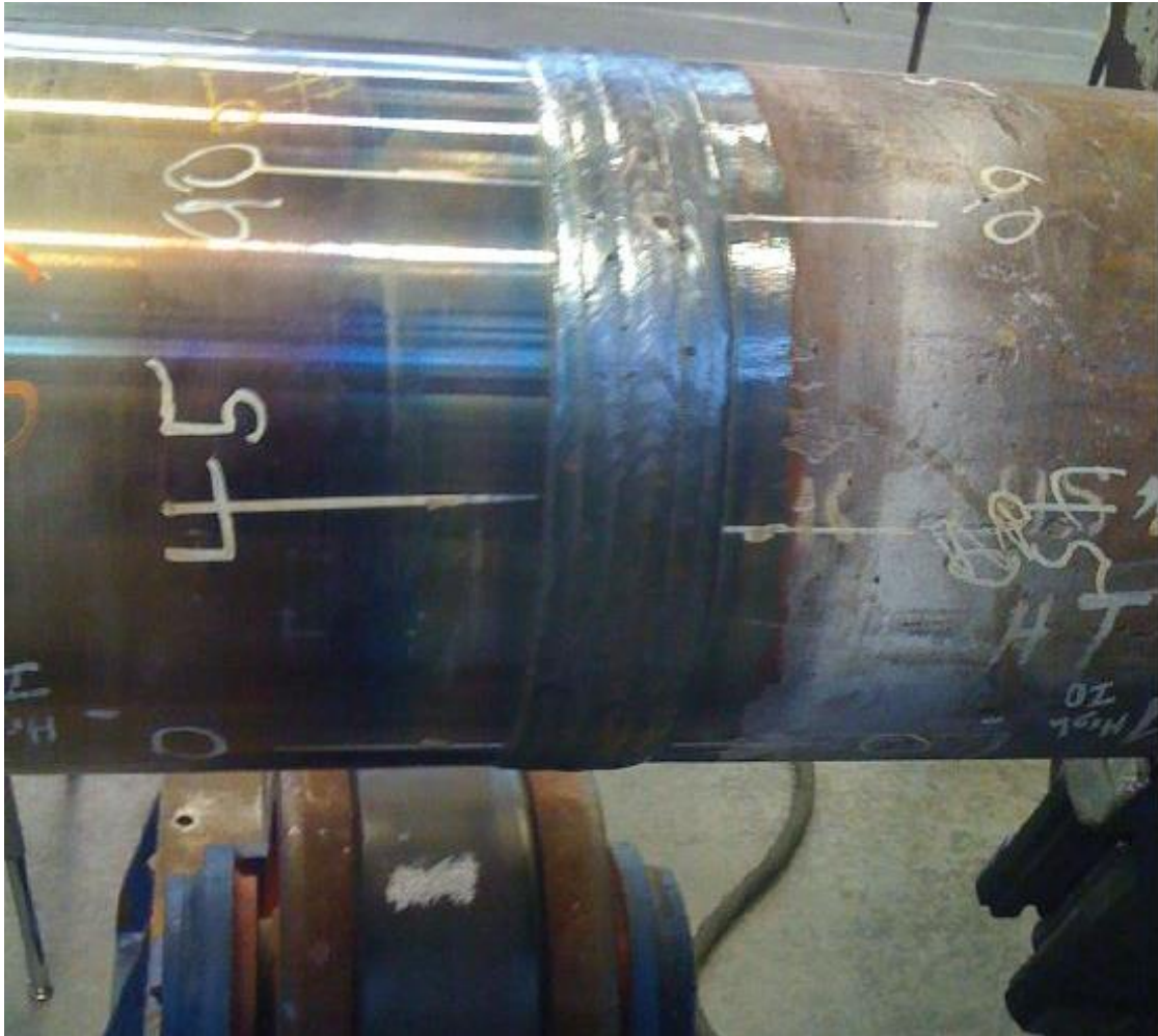
Figure 4.5. Pipe welded with SAW completely (Singh, 2021)
