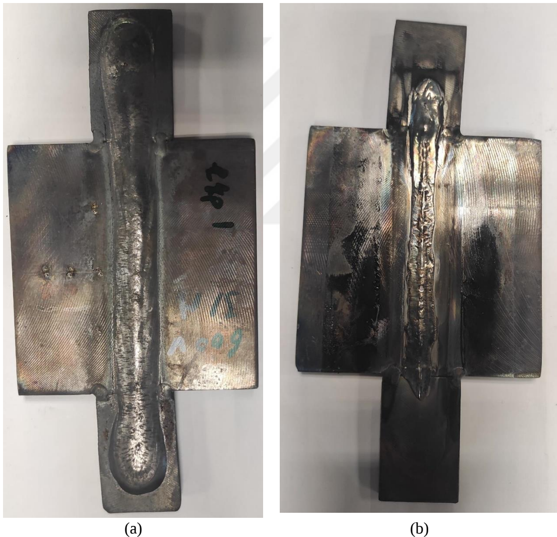
Figure 6.2. (a) Top face of the welded part (b) bottom face of the welded part
