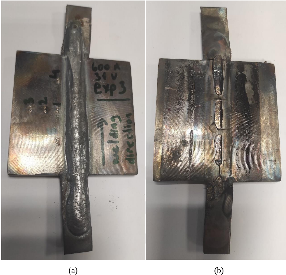
Figure 6.3. (a) the top face of welded part (b) the bottom face of welded part
