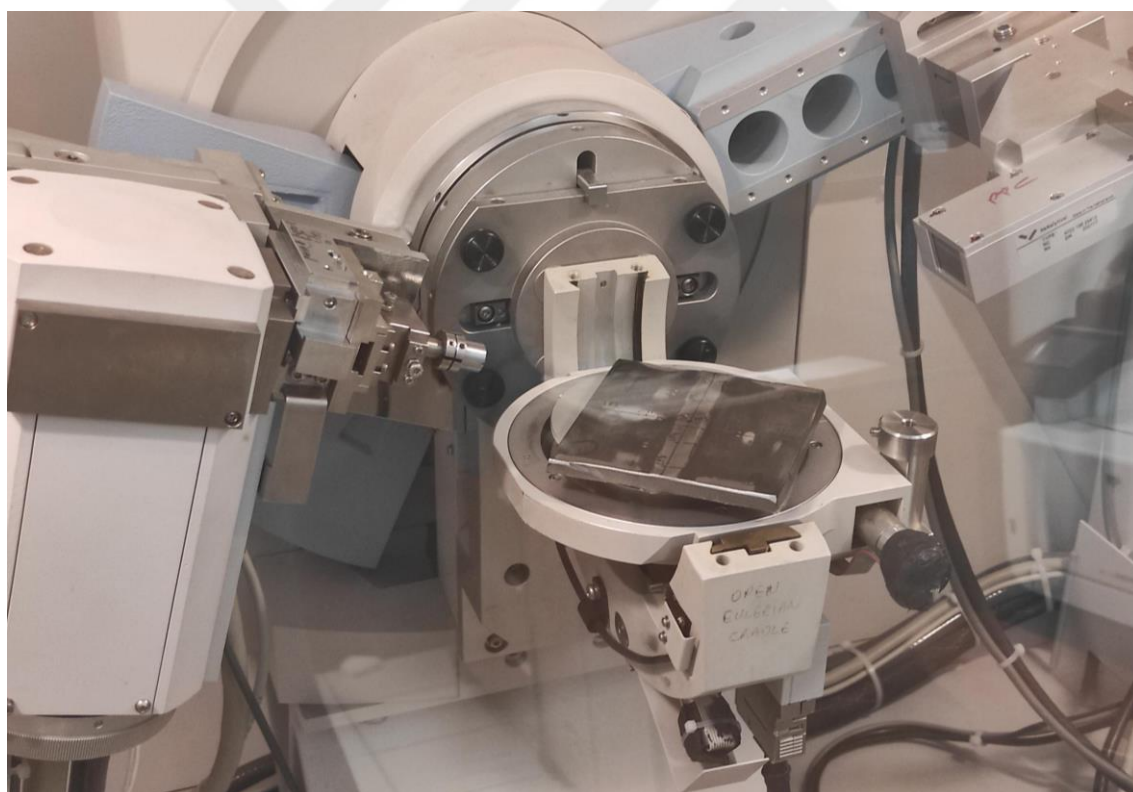
Figure 6.34. The part located to X-pert Pro MPD
