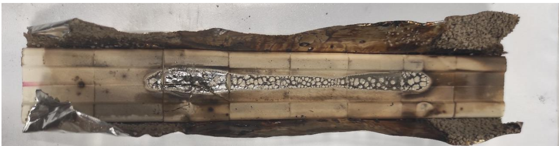
Figure 5.7. The view of ceramic protector after welding process
