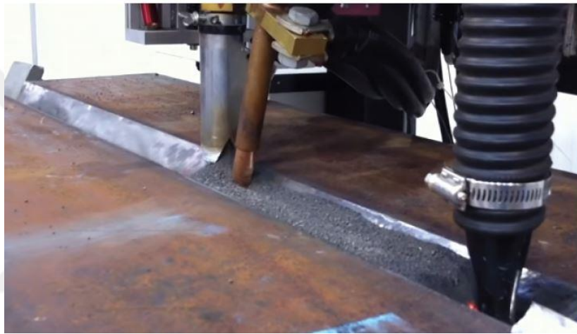
Figure 4.3. Flat plate welded with SAW (Singh, 2021)
