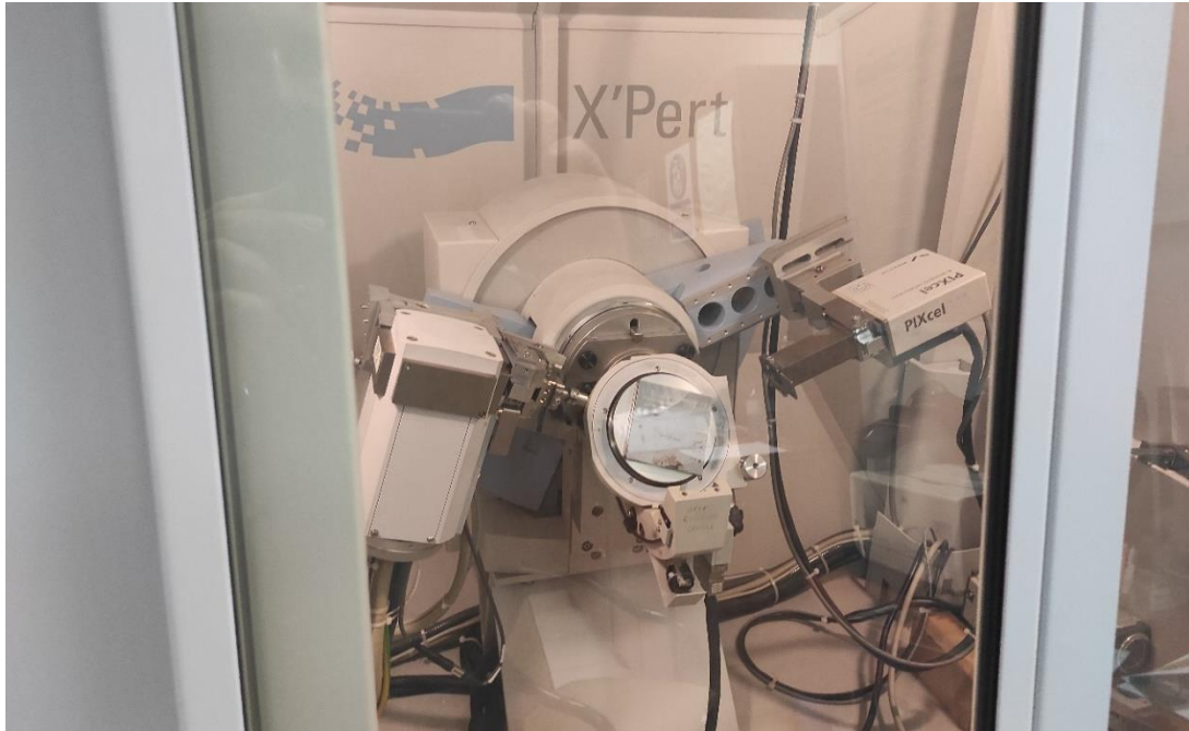
Figure 5.18. Measuring of residual stress on welded part
