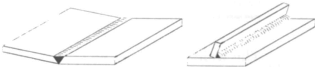
Figure 2.1. Distortion caused by welding (Croft D.N., 1996)
