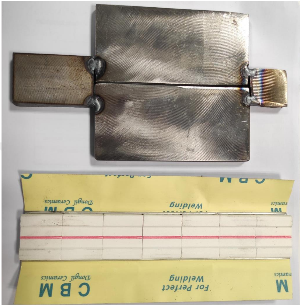
Figure 5.6. Setup of test plate for SAW
