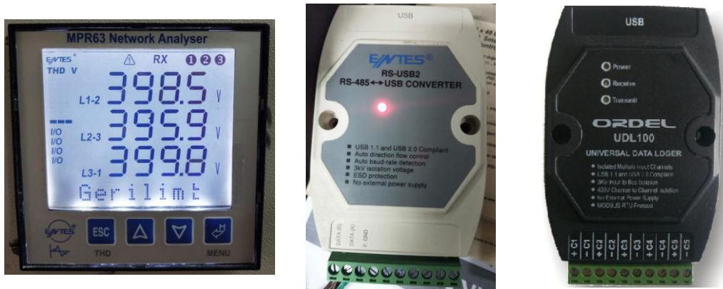
Figure 3.11. Photographs of the network analyzer (left), RS485-USB converter (middle), and the universal temperature data logger (right)
