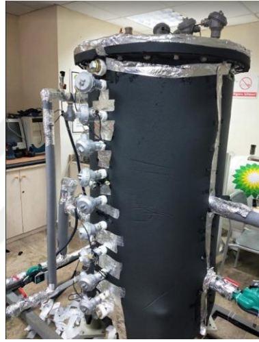
Figure 3.9. Photograph of the thermal energy storage tank with insulation and thermocouples
