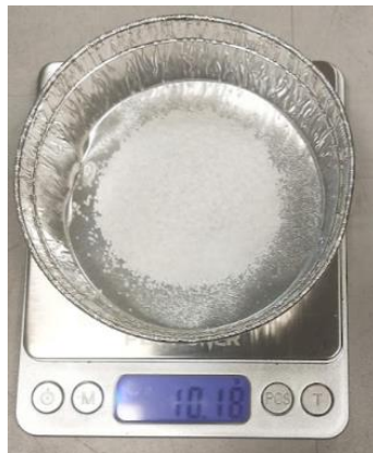
Figure 3.17. Lauric acid in granular form before DSC tests
