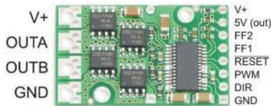
Figure 3.31. Top view of the MOSFET H-Bridge High-Power Driver 30v15
